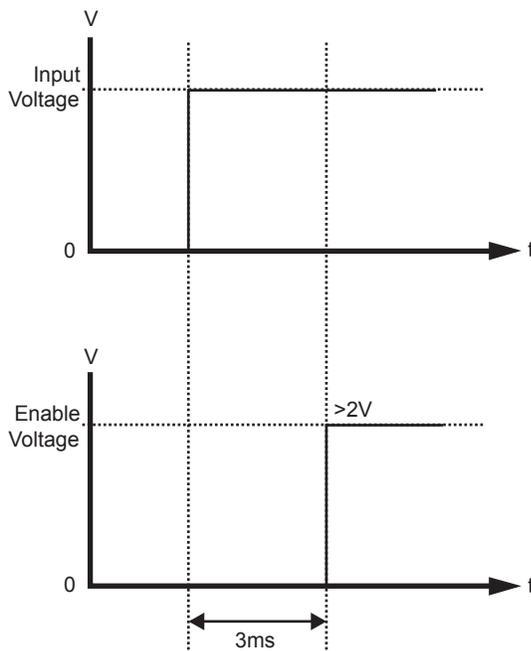
**Figure 2—Input Voltage vs. Enable Sequence**
